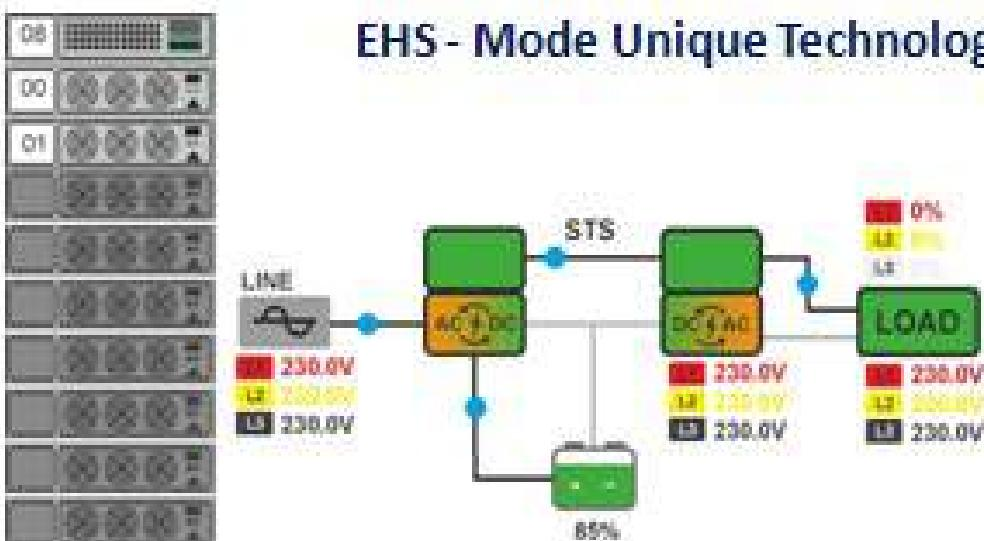
**EHS mode (Efficiency  $\geq 98.4\%$ )** – Inverter as well as Rectifier are in fully ready state and in sync with load and mains power to ensure the power transfer to inverter / battery mode instantly.
