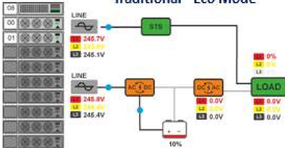
**ECO mode (Efficiency  $\geq 99\%$ )** - Mains power
