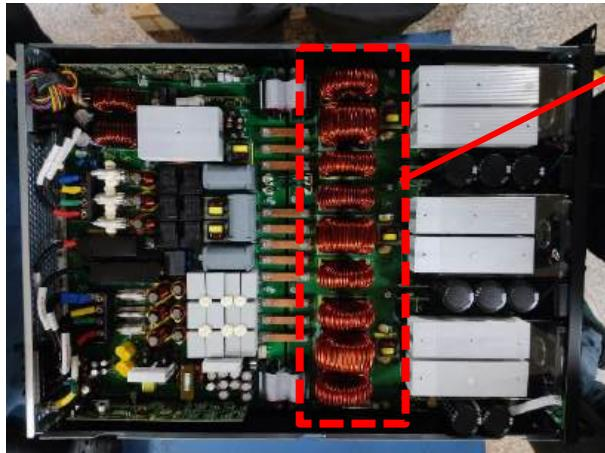
Vertical arrangement of coils
